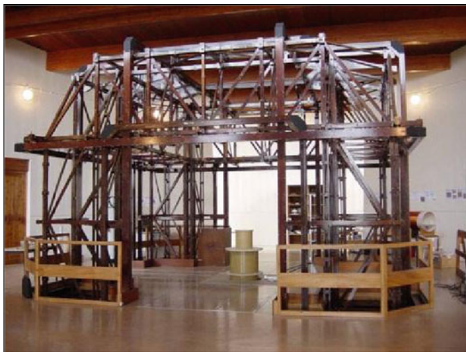
Fig. 13.7 6.6 m coil facility at CNES (image: CNES)
